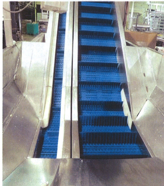
Figure 28. The dual conveyor belt picks up fish in small and large increments, to be used to fill the hoppers to the desired weight for packaging.
