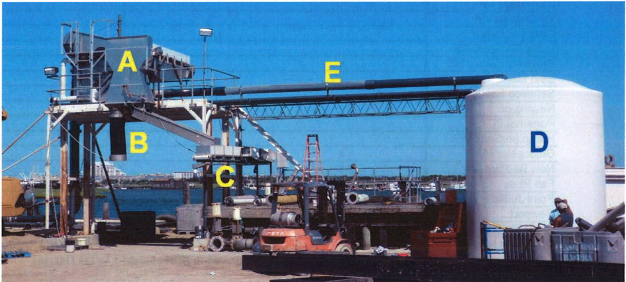
Figure 23. The herring, after pumped off the boat and to the de-watering box (A) are then either deposited into trucks or poultry bins via a hose for bait sales (B) or into the facility via a conveyor belt (C) and then into tubes into the plant for the food market. Meanwhile cold water is re-circulated between the boat and the storage tank (D) via pipes (E).
