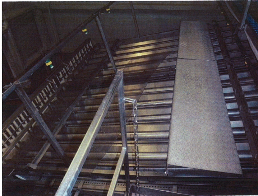
Figure 26. A sorting machine in which different sized herring fall to different levels depending on their ability to fit through the bars.
