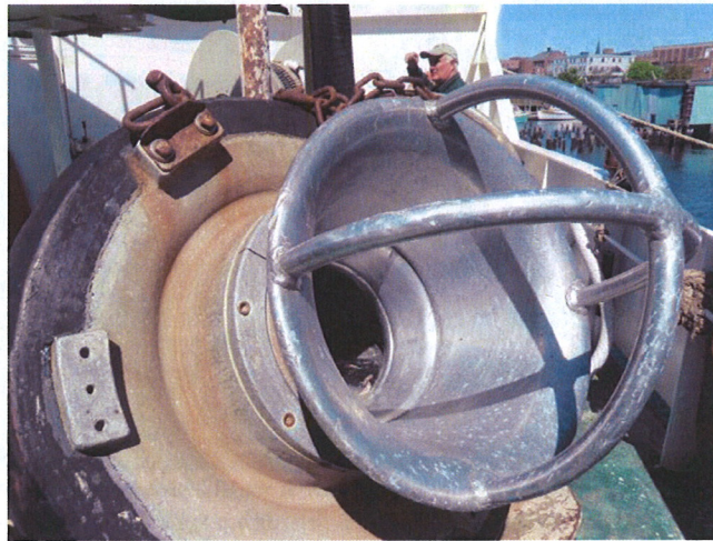
Figure 1. A bell, the beginning of the pumping process on a herring vessel
