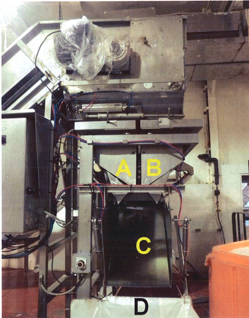
Figure 29. Each of the two hoppers pictured here (A and B) has an electronic scale to verify the total weight of the fish. As one hopper opens to drop the fish down the chute (C) and into the packaging (D), the other hopper is being filled and the contents weighed and later opens as the first hopper begins to fill again.
